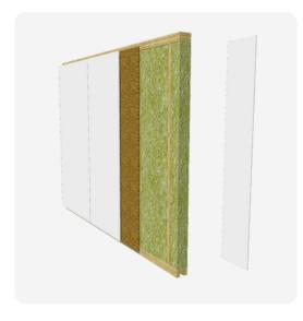
Gypsum plasterboard, 12.5mm Wood based board, 12mm Structural frame, 95-145x45mm Thermal insulation, 95-145mm Gypsum plasterboard, 12.5mm
