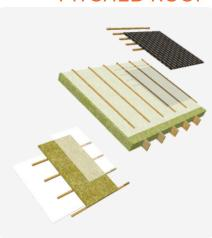
Roof covering (Concrete, Ceramic, Steel, Composite tiles) Solid wood battens, 45x45-60mm Solid wood battens, 45x45mm Bitumen/polymer reinforced sheets Wood based board, 18-22mm Solid wood battens, 45-95x45-60mm
